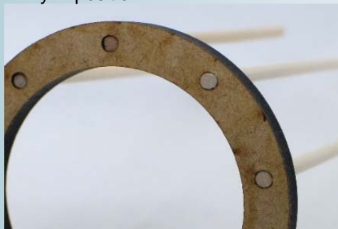
5. Each rod should be as flush as possible with the base.
